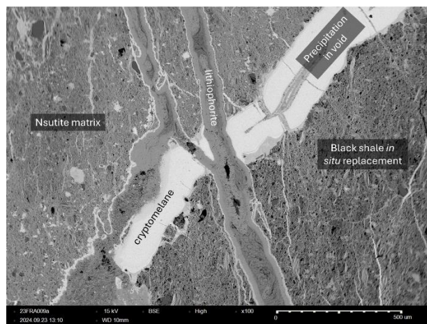
Figure 6. Petrogenetic relations in the platy Mn ore of the Franceville Mn-rich regolith (SEM view under BSE mode).
