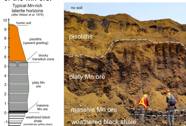
Figure 2. Typical structure of the Franceville Mn-rich regolith in the Kouma mine (Comilog-Eramet, 2023).
