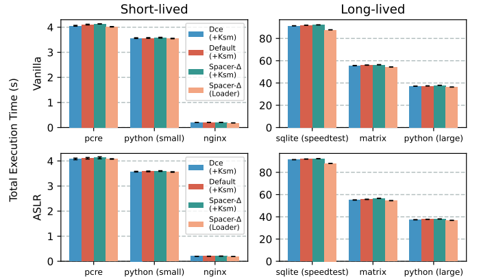
Fig. 10. Total execution time of several applications/versions using five different versions of a specific library, executed in standalone mode. Spacer- \Delta configuration, combined with a custom loader, yields the best performance.
