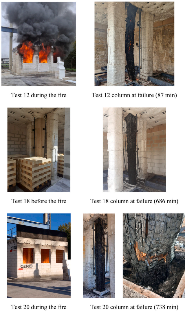
Fig. 8. Pictures of three of the compartment fire tests on glulam columns.
