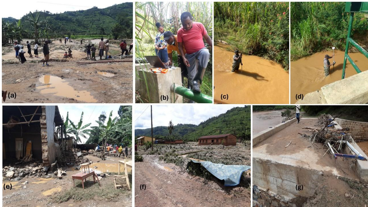
Note: (a, e) flood events in the Nyamutera catchment; (f) flood depth; (g) destruction of the Rubagabaga small bridge; (b) downloading TD-Diver data at the Nyamutera hydrometric station; (c, d) flow measurement using a current meter; (d) surveying a cross-section of the Gaseke River.
