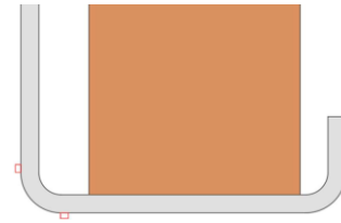
Figure 4 Position of the strain gauges indicated with red squares
