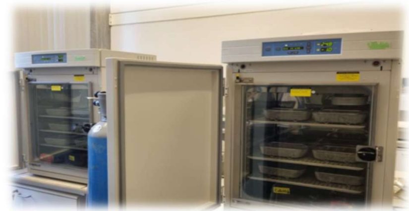
Static carbonation chambers
