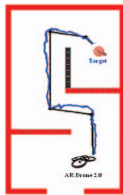
Fig. 14. Real-time obstacle avoidance of the AR. Drone 2.0 with pattern-based localization, MPFM and PD controller.
