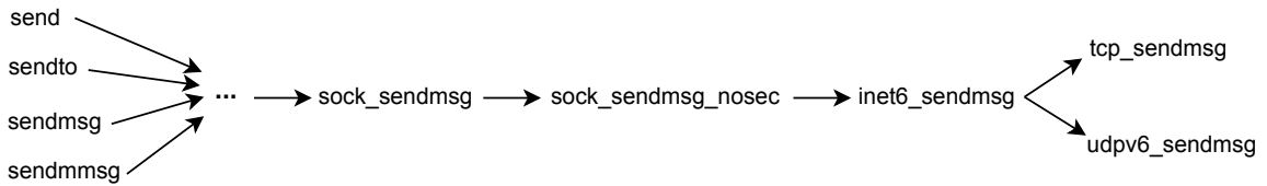
Figure 12.1: Call graph of send system calls for IPv6 and Layer-4 in the Linux kernel.
