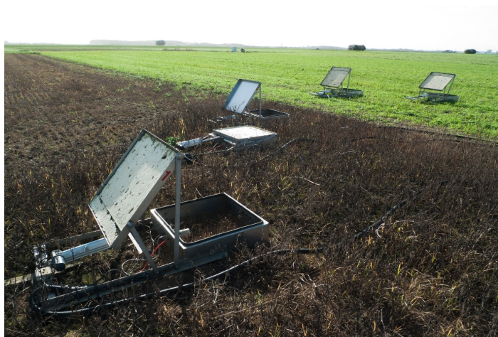
Figure 3.1 – Field view showing residue returned to the soil after crop harvest, together with the automatic chambers used for measuring N 2 O emissions (Photocredit: Joël Léonard).
