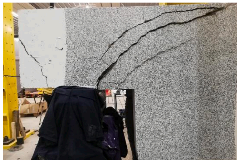
(b) Shear failure (specimen DL8 [18])
