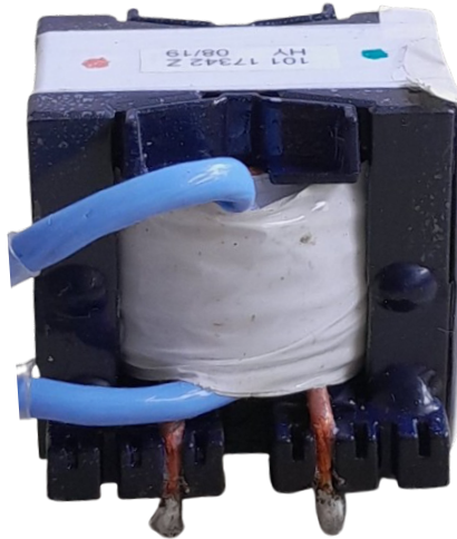
Figure 5.10: Resonant transformer used in the LLC converter.
