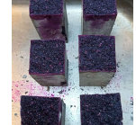
Figure 3: Concrete blocks made with carbonated MSWI-BA
