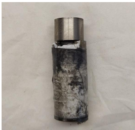
Figure 2.4. Freshly extracted 3/4" assembly after quenching an experimental run. The assembly is wrapped in PTFE (greyish film) and covered in a mixture of mineral oil and MoS 2 (or molikote, dark stains on the PTFE sheet) to facilitate the assembly extraction from the pressure vessel of the piston-cylinder. The steel plug for the thermocouple insertion can be seen on the top of the image (the pyrophyllite ring encircling the steel plug is missing).
