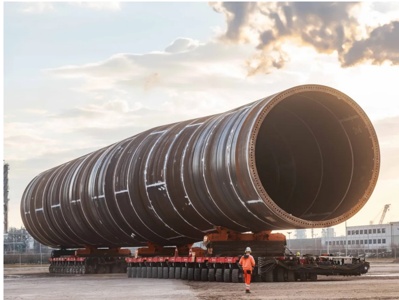
Fig. 1.2 A fabricated monopile for an offshore wind farm [8]. The alternating light and dark bands reveal the individual rolled steel cans that are joined by circumferential welds. This underscores the number and scale of potential fatigue hotspots in a full-size monopile structure.
