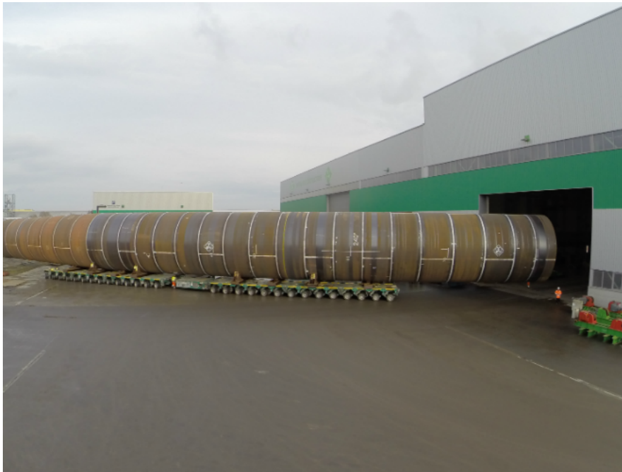
Fig. 2.1 A typical large-diameter monopile fabricated for an offshore wind farm in the German North Sea [69]. The alternative light and dark bands reveal the individual cylindrical sections formed by rolling steel plates, which are then joined by circumferential welds to achieve the full length of the monopile.
