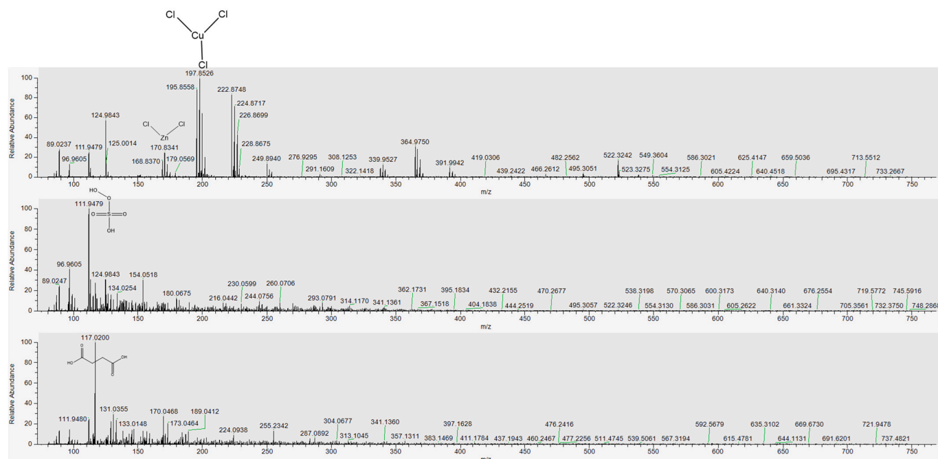
Fig. 5. The mass spectra (negative ionization mode) from the Direct Analysis in Real Time coupled to High-Resolution Mass Spectrometry analyses of nitrile gloves. The top figure represents new gloves, while the middle and bottom figures depict 18 months sea and sand aged nitrile gloves, respectively.
