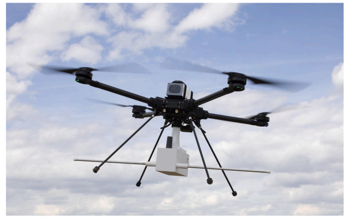
Fig. 2. Drone-borne GPR system. The platform is a Tundra drone (Hexadrone, France), carrying the gprSense® prototype (spring 2023 version, Sensor Consulting, Belgium). The white enclosure houses the battery, micro-computer, and VNA, and the 1-m dipole antenna rods are fixed to the front lower part of the enclosure.
