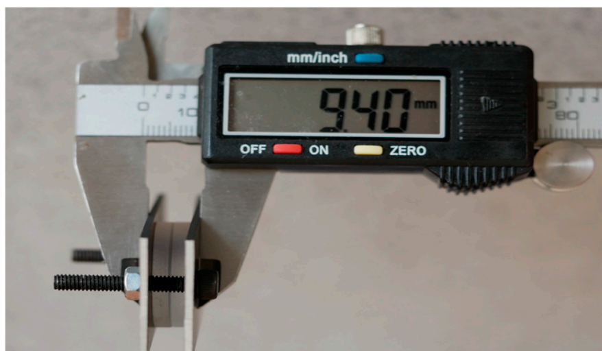
Figure 3. Measurement of tissue sample thickness using calibrated electronic micrometer.
