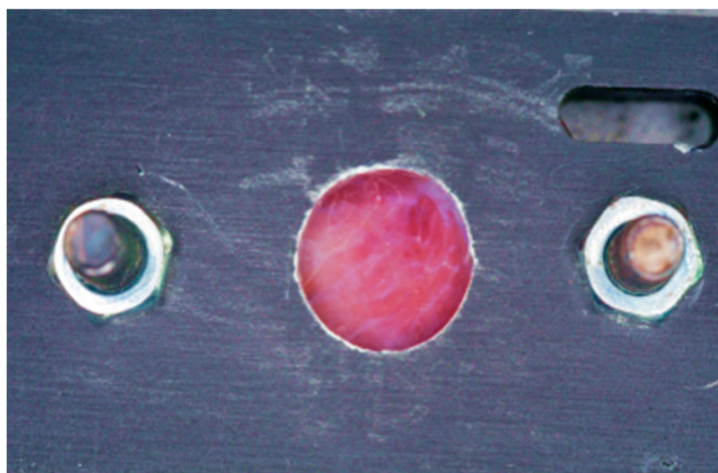
Figure 2. Tissue sample positioned between two FOCtek optical glass slides within a custom metal stabilization device.
