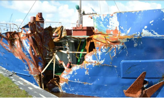
Figure 2. Cargo ship Petra L. stroke an offshore wind turbine at Gode Wind 1 wind farm (Germany), 2023 - From (Offshore-energy.biz, 2023)
