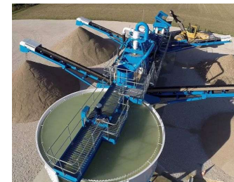
Washing + air separation
