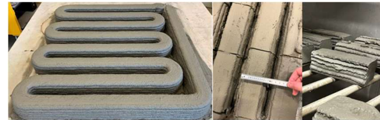
Printed samples (4x4x16 cm prismatic samples extracted from S shaped printed elements)
