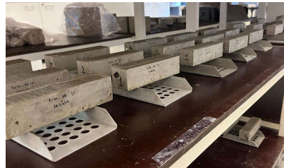
Casted samples (4x4x16 cm prismatic samples)
