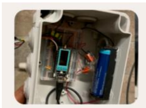
Figure 5. Creation of a PiLowTech irrigation sensor during a highlow tech session
