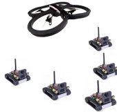
Fig. 2. Proposed formation control scheme using UGV SRV-1 robots and one UAV as remote vision sensor.
