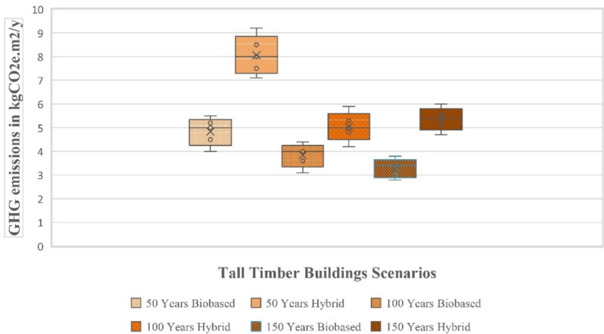
Fig. 2 Comparative bar chart illustrating the greenhouse gas (GHG) emissions for biobased-only construction versus hybrid construction with steel and concrete consolidation over 50, 100, and 150 years
