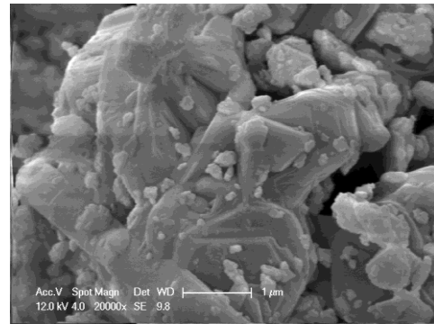
Fig. 2. SEM image of \text{Ba}_{0.5}\text{Sr}_{1.5}\text{Zn}_2\text{Al}_{0.08}\text{Fe}_{11.92}\text{O}_{22} powder.
