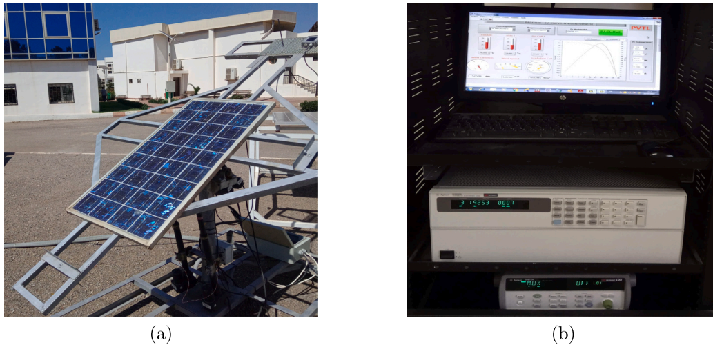
Fig. 1. Characteristics of the deployed PV module sample: (a). outdoor mobile structure for solar tracking. (b). Software and hardware for PV curve tracing (I-V and P-V).
