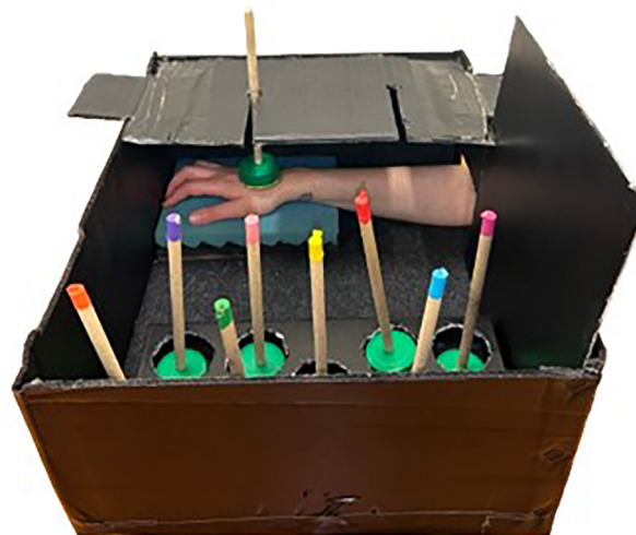
Fig. 1 – Stimulation box. The box has two openings to insert the right and left arm. Two holes on the top assure that the stimulus is slid on the proper area. The 9 stimuli are formed by a wooden stick attached to a cork, containing the stimulus material inside. To allow the experimenter selecting the type of stimulus, without recognizing its identity, a colour cap was inserted on the top of each stick.
