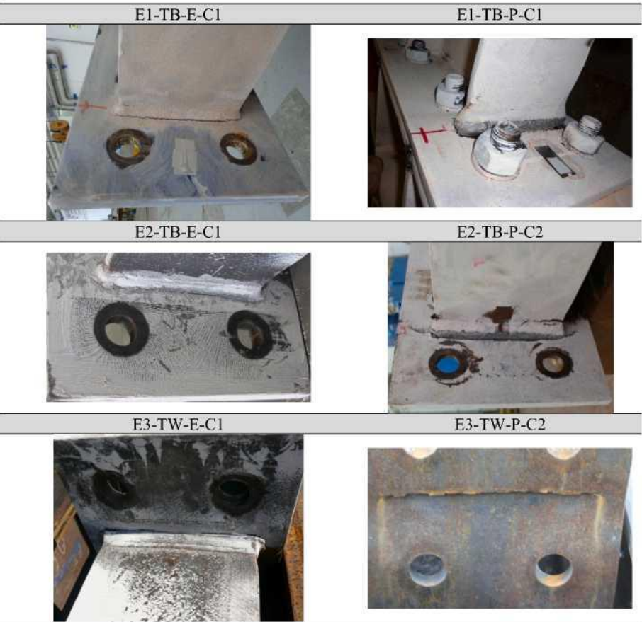
Fig. 9. Pattern of cracks in the damaged joints at the end of the tests (i.e., for E1, E2 and E3 after the constant amplitude cycles at the maximum stroke of the actuator).
