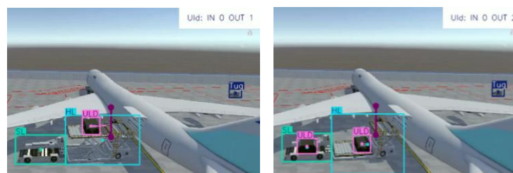
Figure 7. Aircraft unloading progress monitoring
