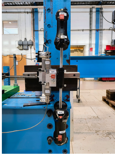
Figure 1. Experimental setup for the whole damper configuration.
