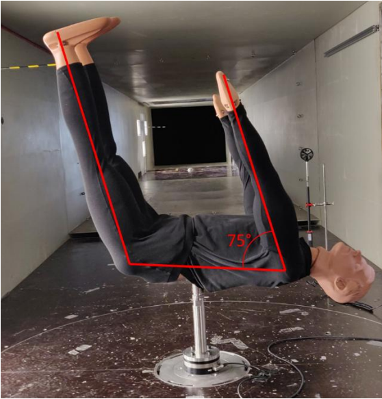
Figure 8: Mannequin in drowned position, tight clothing and yaw angle of 90°. Articulations blocked to have limbs with an angle of 75° with the horizontal.
