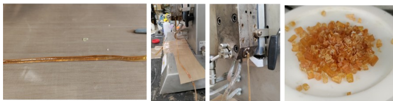
Figure S2.38. Filament produced from the twin screw extruder and pellets (T_S6).
