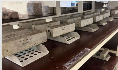
Casted samples (4x4x16 cm prismatic samples)
