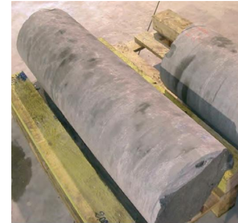
Borehole core samples (Andra, 2005)
