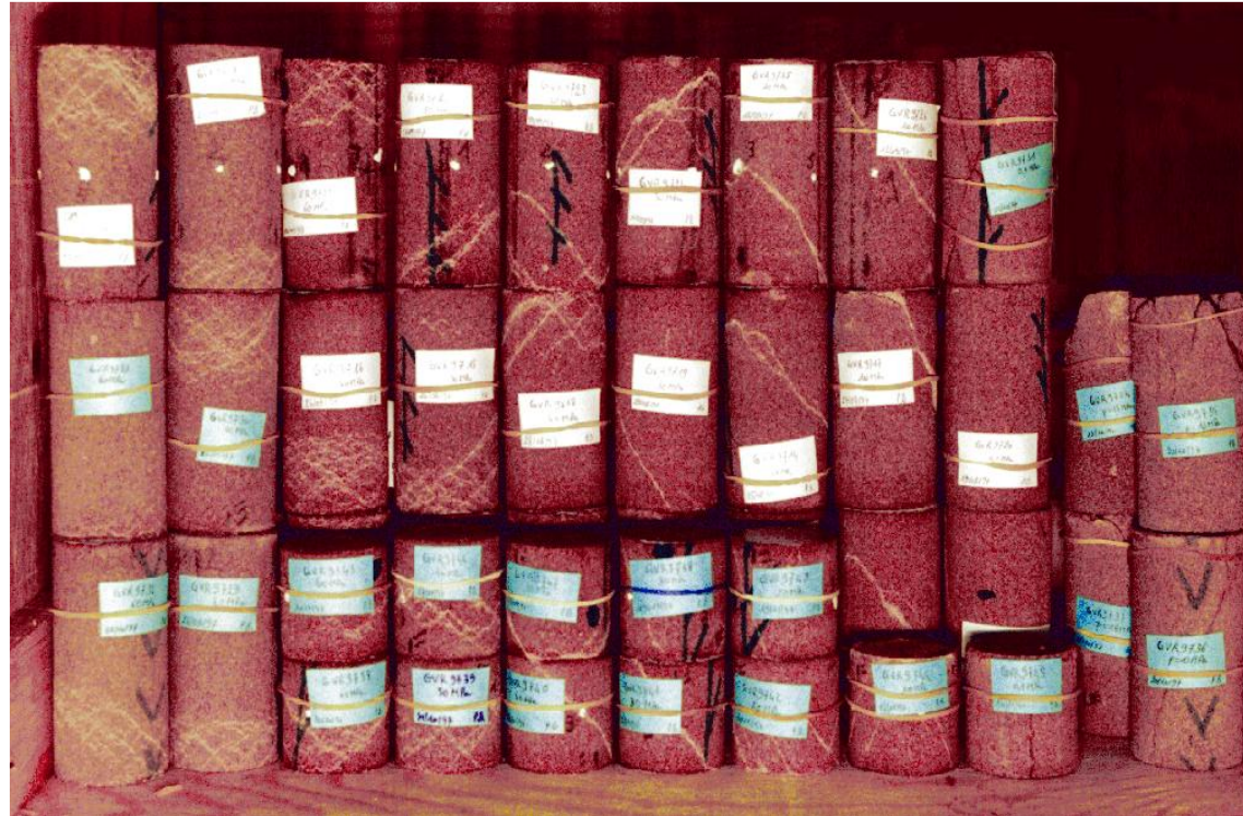
Localized rupture in sandstone samples under different confining pressures (Bésuelle et al., 2000)
