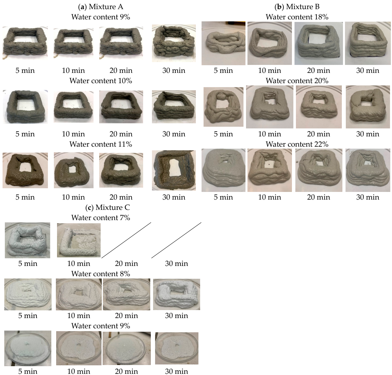
Figure 8. The pistol test results: (a) Mixture A with 9, 10, 11% water content; (b) mixture B with 18, 20, 22% water content; (c) mixture C with 7, 8, 9% water content.
