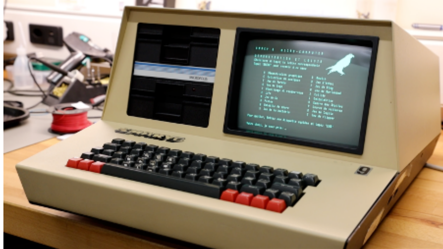
A Smaky 6 computer (1978–82)—a beige solid box with two floppy drives and a monitor—running a floppy disk with games and demonstrations (Photograph by Prof. Yannick Rochat, October 24, 2023) (Courtesy of the author)
