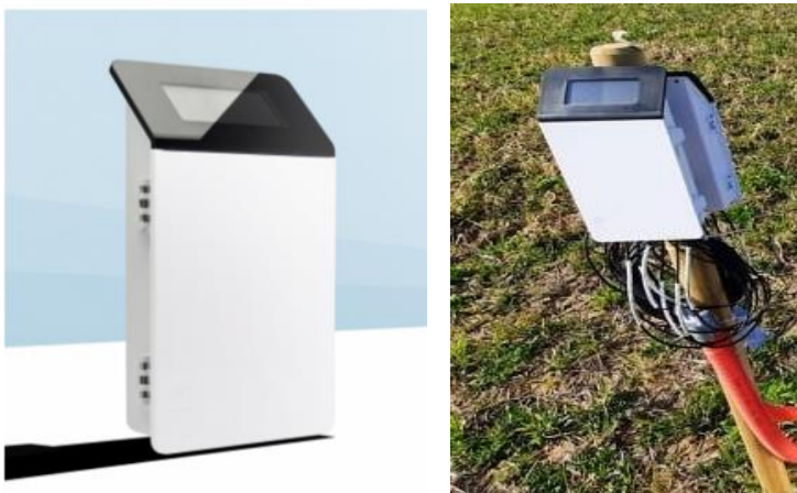
Figure 14. ZL6 data logger from MeterGroup with integrated solar panels
