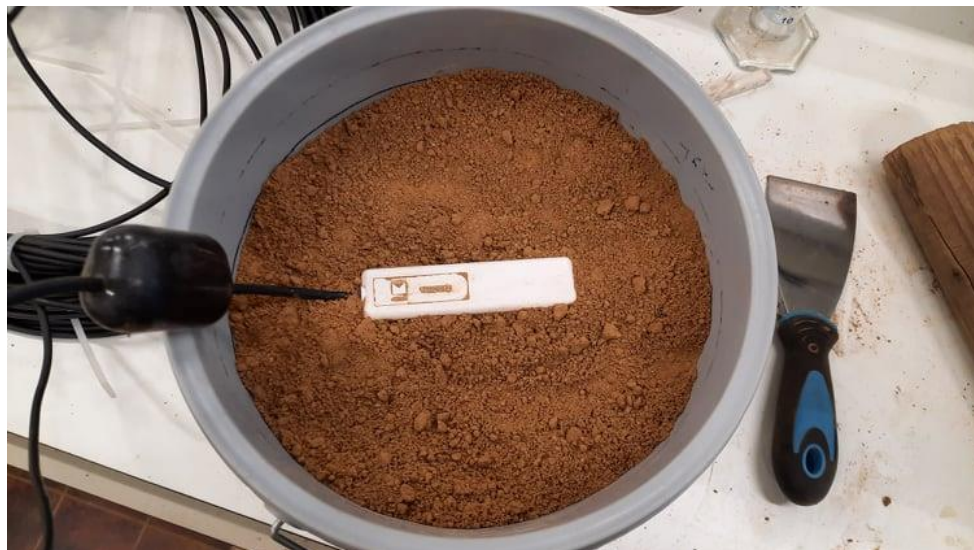
Figure 27. Calibration of a Teros 12 sensor.
