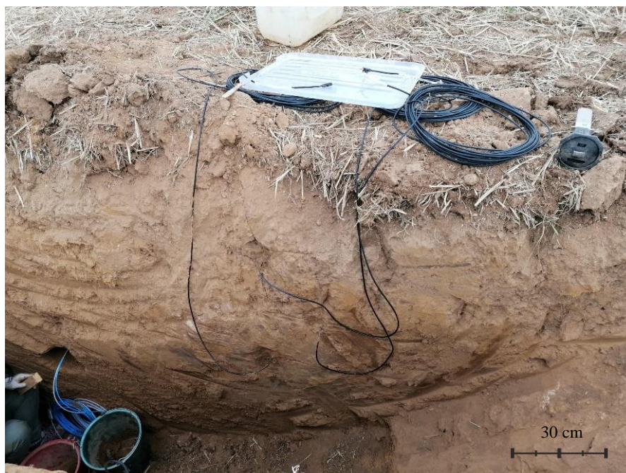
Figure 10. Soil profile during installation of hydrological monitoring equipment
