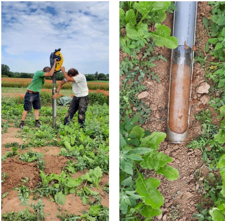
Figure 32. Sampling of intact soil columns up to 30cm depth with the gasoline-powered percussion hammer.
