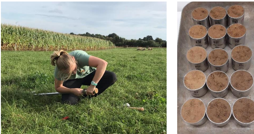
Figure 49. Sampling of the soil bulk density and preparation in the laboratory
