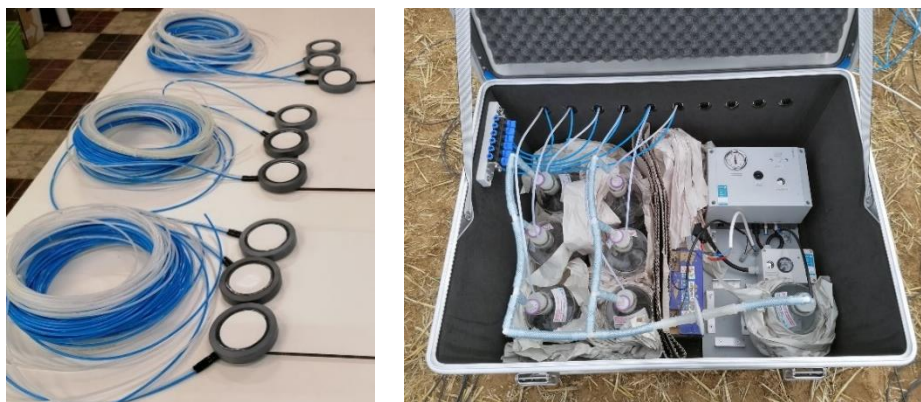
Figure 15. EcoTech glass sampling plates with its isothermal storage box containing the vacuum pump, sampling bottles and battery.
