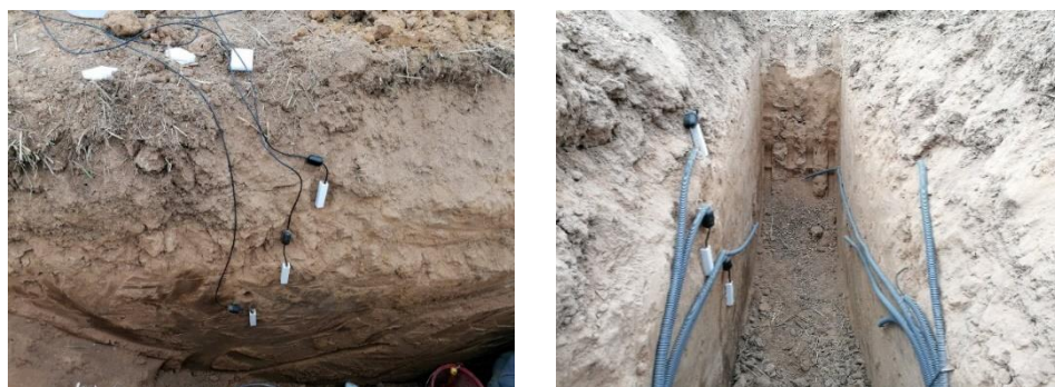
Figure 18. Installation of Teros 12 and Teros 21 sensors in parallel in a trench on a plot at a depth of 30, 60 and 90 cm.
