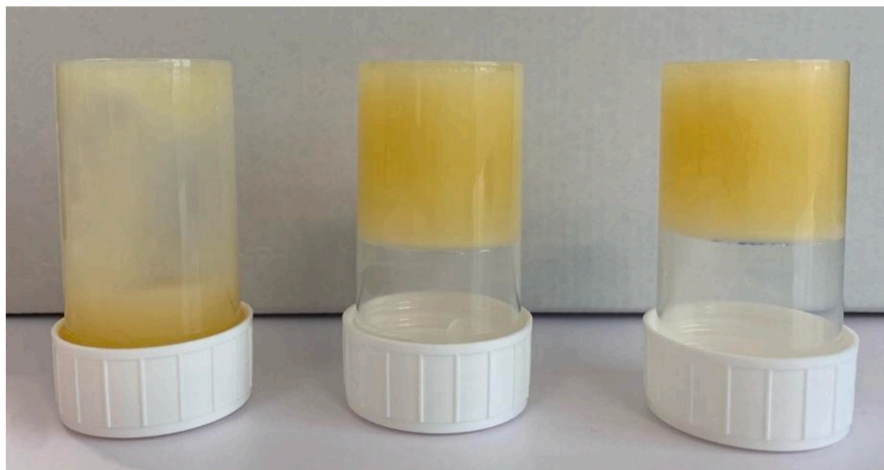
Fig. 1. Minimum concentration of waxes necessary to visually self-structure the oleogel. Carnauba wax example, from left to right, 4.0, 4.2 and 4.4 % (w/w) of wax in rapeseed oil.
