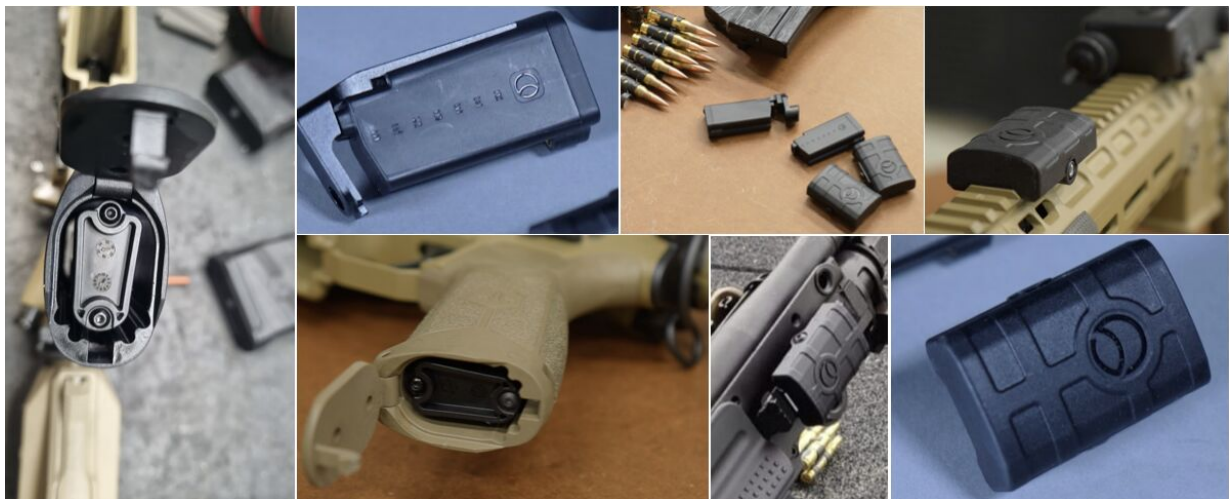
Figure 1.18: WeaponLogic devices by Senseer. These are accelerometer-based, and rely on an undisclosed machine learning to produce their shot counting algorithm [12].
