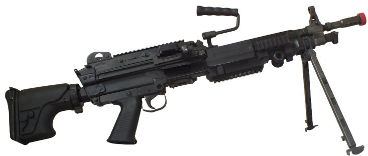
(b) Blank-firing adaptor affixed to a FN Minimi.
