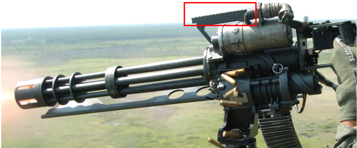
Figure 4.16: M134 Minigun. The standard (Picatinny) accessory rail is highlighted in red.
