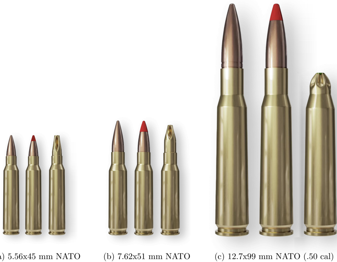
Figure 1.25: Types of ammunition used in this study. Each calibre features from left to right: a standard live cartridge (“ball”), a tracer round, and a training round (“blank”).
