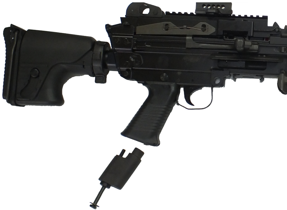
Figure 1.17: FN SmartCore ® device embedded in a standard machine gun grip. The only mechanical modification needed is a lengthening of the screw that normally affixes the handle to the lower receiver to also affix the shot counter.
