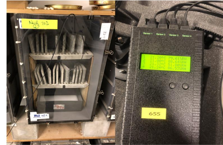
Figure 4.3: Left: Chambers used for the static sorption and desorption experiment, with the RH and temperature probe and the samples inside. Right: sensor housing displaying the measures for the four probes used.
