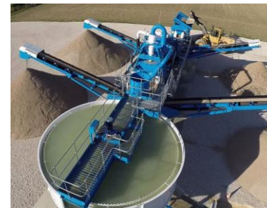
Washing + air separation
