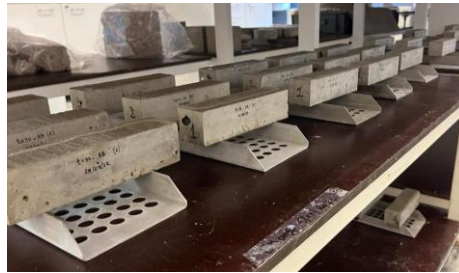
Casted samples (4x4x16 cm prismatic samples are casted)
