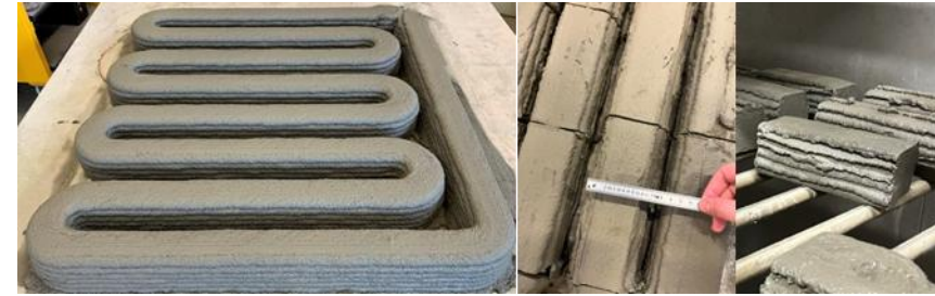
Printed samples (4x4x16 cm prismatic samples are extracted from S shaped printed éléments)
