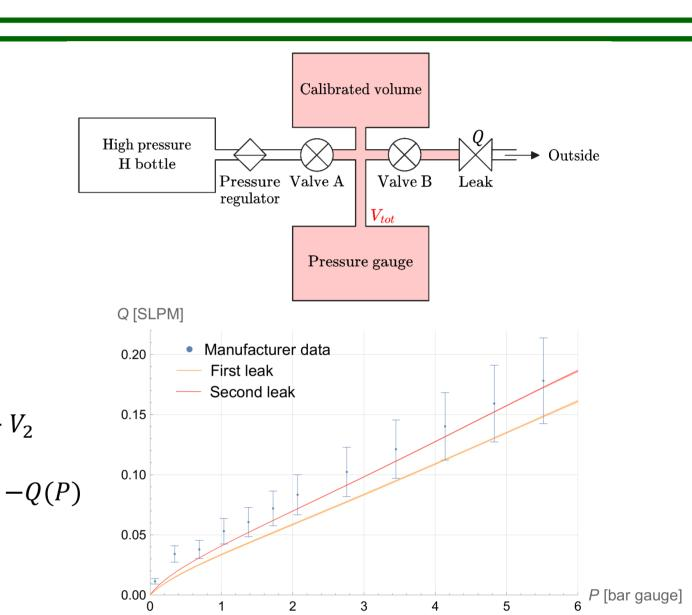
Leak rate calibrations for both leaks used during the experiments
