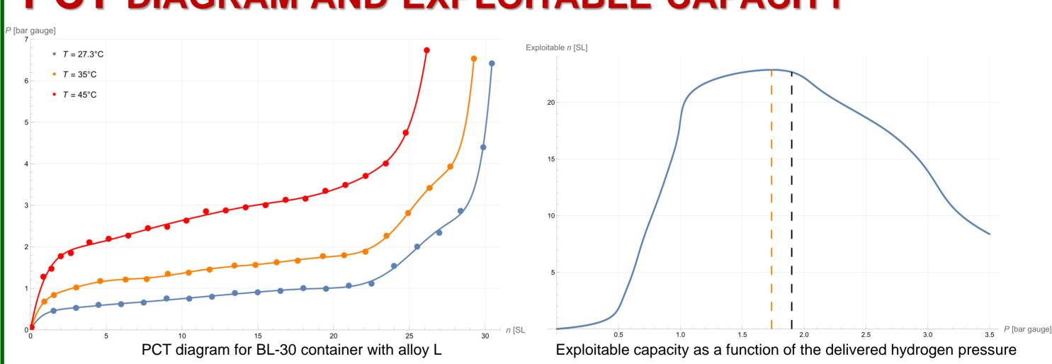
Maximum exploitable capacity: 22.9 SL at 2.7 bar absolute
