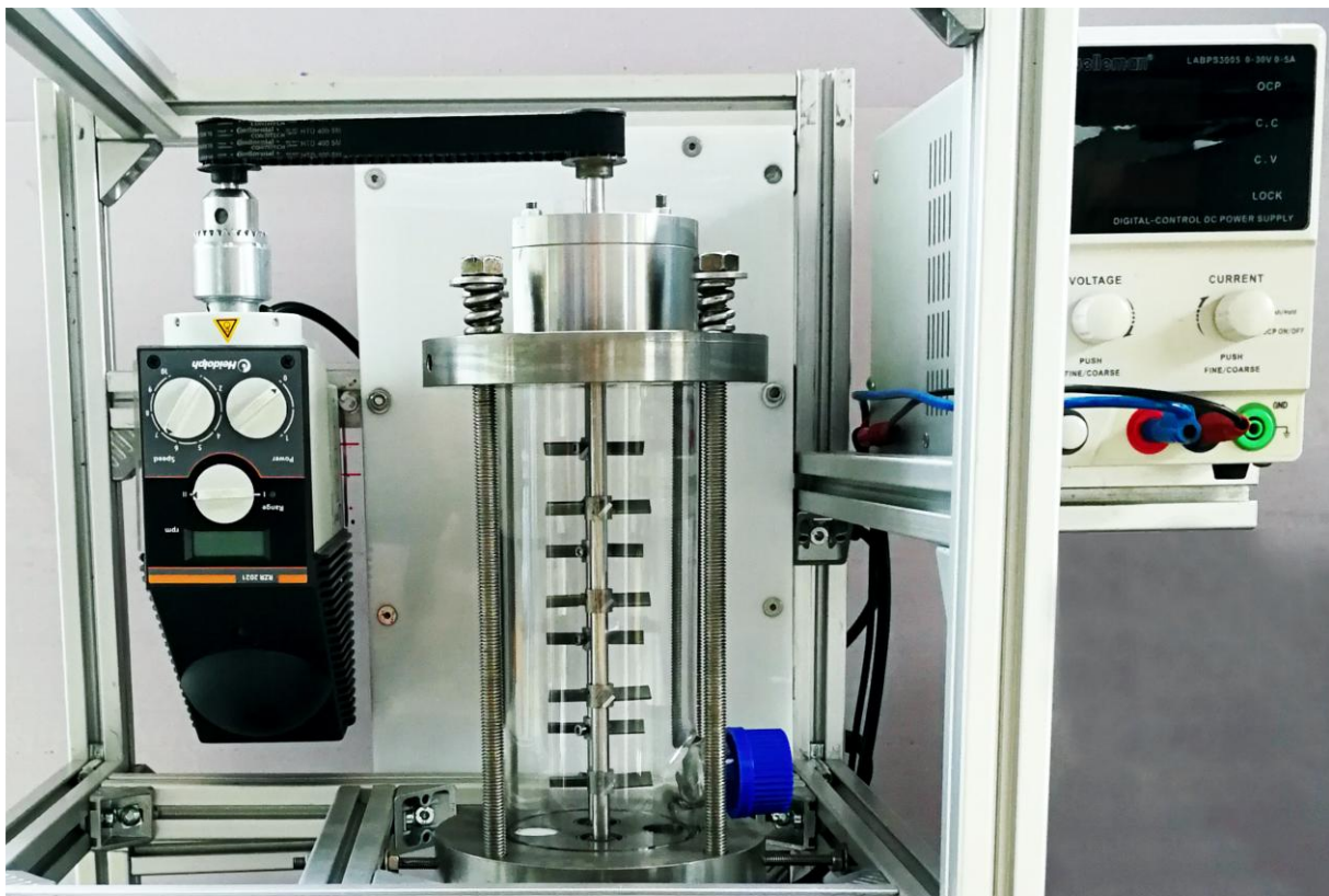
Fig. 6-8: Optimized settling cell based on Henschke's standardized stirring-cell design
