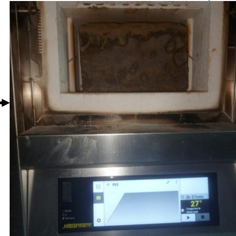
Box placed in the muffle furnace at 950°C for 3 hours
