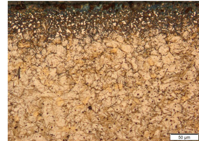
Chemical treated bio-carburizer: carbides, retained austenite
