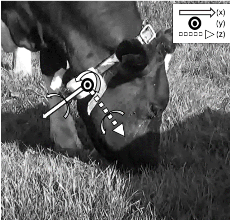
Figure 5-2: Wearable IMU and GNSS sensor fixed on the collar of the cow. The three coordinate axes of the accelerometer are displayed, and rotation arrows indicate the gyroscope rotational axes.
