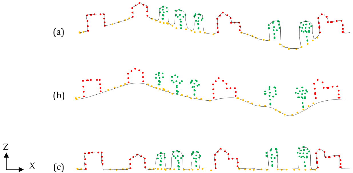
Figure 5. Schematic diagram to show the difference between: (a) DSM (Digital Surface Model), (b) DEM (Digital Elevation Model), and (c) The nDSM (normalized Digital Surface Model).
