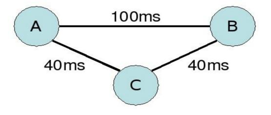
• It is possible to obtain a better latency gain by using more than one intermediate node as alternative path (future work).
