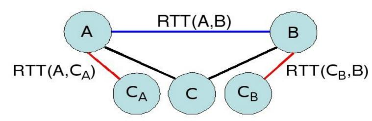
• If  $RTT(A,C_A) + RTT(C_B,B) < RTT(A,B)$  then C is considered as a shortcut for the link AB.
