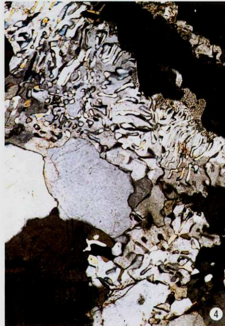
1. Quartz monzonite; clinopyroxene alteration to hornblende (central left); evidence of deformation in quartz and biotite (upper right); typical structure of titanite growing on ilmenite (black, lower left); crossed polars, x 28, Goldap 4, depth 1648.0 m. 2. Granodiorite; titanite growing on ilmenite (black); numerous biotite slightly altered to chlorite; plane polarized light, x 28, Goldap 2, depth 1636.5 m. 3. Quartz monzonite; large K-feldspars and plagioclase, smaller clinopyroxene altered to hornblende (center); plane polarized light, x 28, Bartoszyce 3, depth 2130.5 m. 4. Granodiorite; myrmekite zone; crossed polars, x 70, Bartoszyce 1A, depth 2141.5 m
