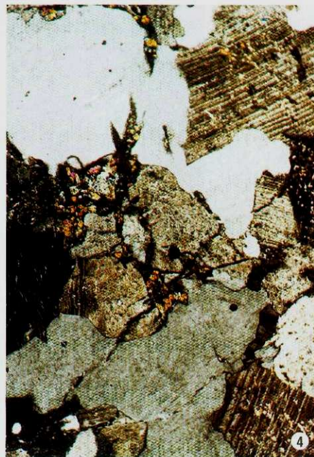
1. Charnockite; main rock components: hypersthene (right center), biotite, quartz, plagioclase; crossed polars, x 28, Łanowicze 10, depth 1162.5 m. 2. Charnockite; hypersthene with numerous inclusions of quartz, ilmenite, biotite and zircon (poikilitic texture); crossed polars, x 28, Łanowicze 10, depth 1162.5 m. 3. Leucogranite; visible microcline and albite crystals, quartz and minute biotite; crossed polars, x 28, Olsztyn 1, depth 2764.0 m. 4. Advanced albitisation and sericitisation of plagioclase with small epidote crystals and xenomorphic quartz crystals; crossed polars, x 28, Olsztyn 4, depth 2780.5 m
