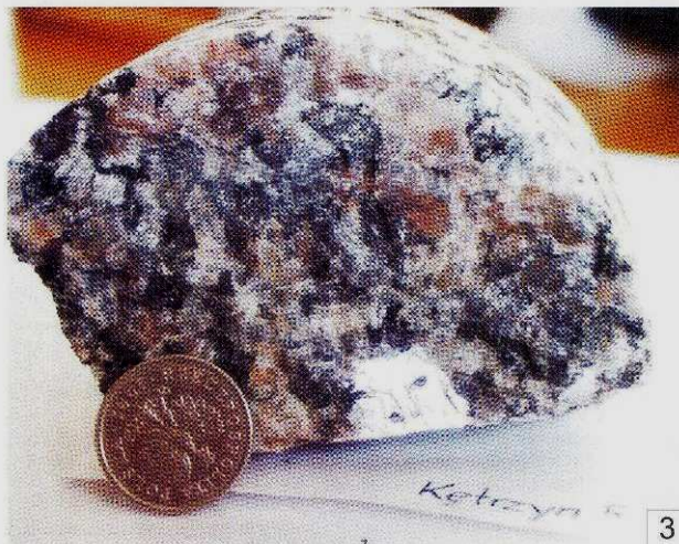
1. Porphyritic texture with large pink K-feldspar in charnockite from the Łanowicze drill-core; depth 1111.8 m. 2. Large plagioclase in quartz monzodiorite from the Filipów drill-core; depth 1553.0 m. 3. Porphyritic texture with large plagioclase crystals in quartz monzonite from the Kętrzyn drill-core; depth 1549.5 m; diameter of the coin is 1.5 cm on all photos
