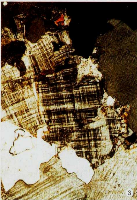
1. Charnockite; main rock components: hypersthene (right center), biotite, quartz, plagioclase; crossed polars, x 28, Łanowicze 10, depth 1162.5 m. 2. Charnockite; hypersthene with numerous inclusions of quartz, ilmenite, biotite and zircon (poikilitic texture); crossed polars, x 28, Łanowicze 10, depth 1162.5 m. 3. Leucogranite; visible microcline and albite crystals, quartz and minute biotite; crossed polars, x 28, Olsztyn 1, depth 2764.0 m. 4. Advanced albitisation and sericitisation of plagioclase with small epidote crystals and xenomorphic quartz crystals; crossed polars, x 28, Olsztyn 4, depth 2780.5 m
