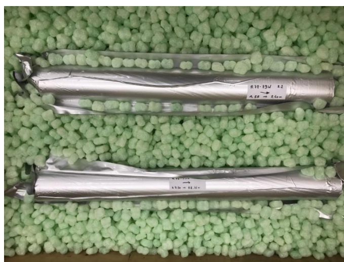
Figure 27 The Boom Clay cores vacuum-sealed in aluminum-reinforced foil.
