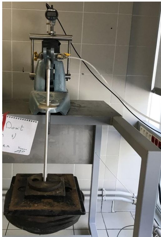
Figure 37 Low pressure oedometer apparatus.
