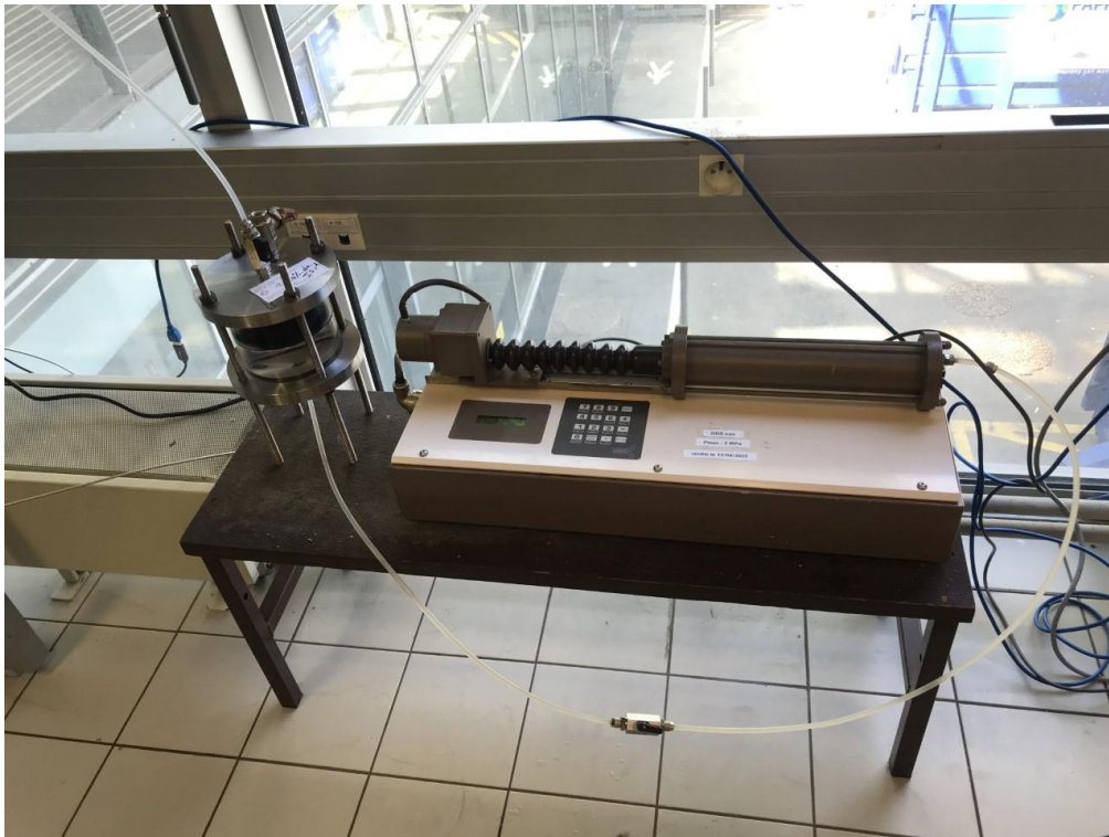
Figure 39 CPV and Interface cell.
