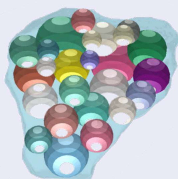
Figure 3. Scan of a rock and its representation with different number of spheres using CLUMP [3].
