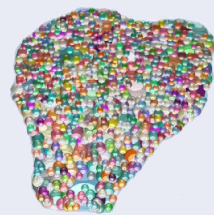
Figure 3. Scan of a rock and its representation with different number of spheres using CLUMP [3].
