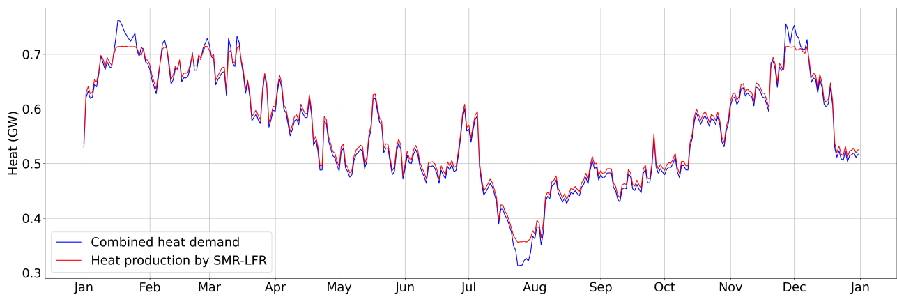
Figure B.10: Representation of heat demand and the heat required for electricity demand, as well as the heat production of the reactor. Representation taken from model H2-AEC (similar to H2-PEM).
