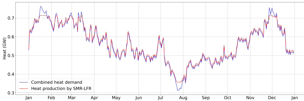
Figure 6: Representation of heat demand and the heat required for electricity demand over a full year, as well as the annual heat production of the LFR-SMR. Representation taken from configuration H 2 -SOEC.
